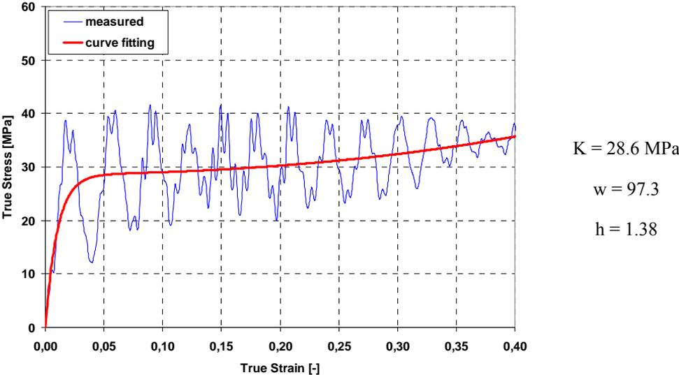
Fig. 3. Comparison of measured and fitting curves with parameters of material model
