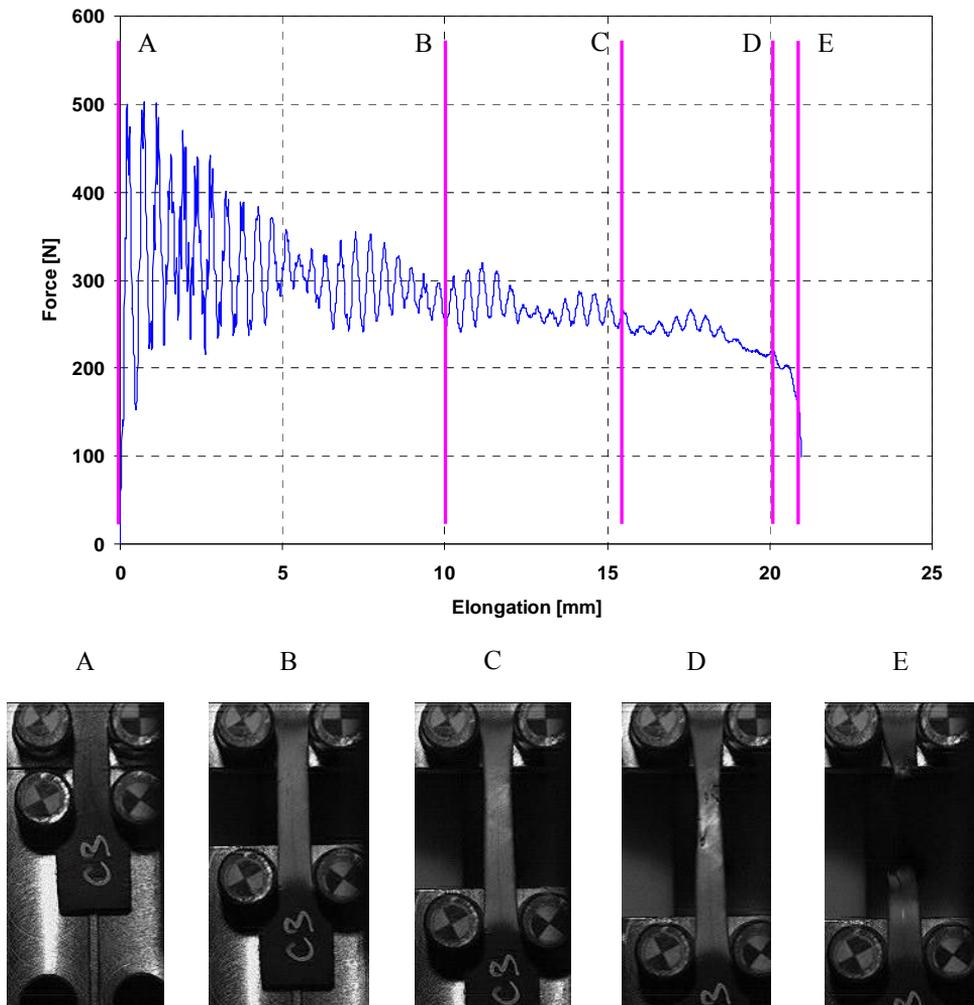
Fig. 4. The measured force-elongation dependence and the hi-speed camera shots
