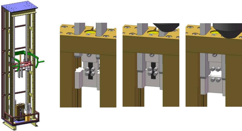
Fig. 2. Full view of the drop tester CAD model and details of the jaws
