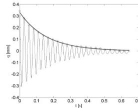
**Fig. 17. Damping curve of specimen №6.**
