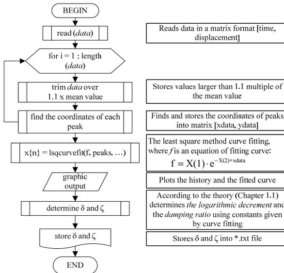
**Fig. 5.** Block diagram of Matlab script.
