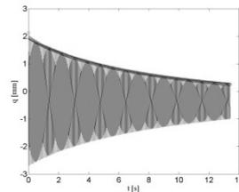
**Fig. 11. Damping curve of specimen №3.**
