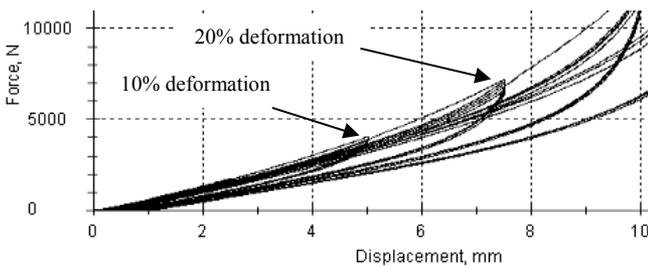
Fig. 2. Viscoelastic behaviour of rubber; Mullin’s effect.
