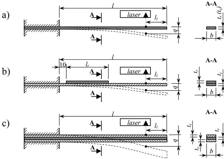
**Fig. 4.** Arrangement of experiments: a) separate rubber/composite
