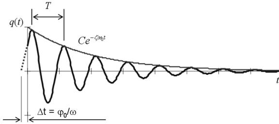
Fig. 1. Response of underdamped harmonic oscillator.
