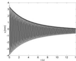
**Fig. 9. Damping curve of specimen №2.**
