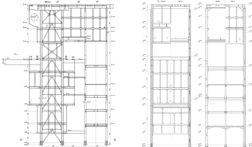
**Fig. 1.** Original boiler supporting structure.
