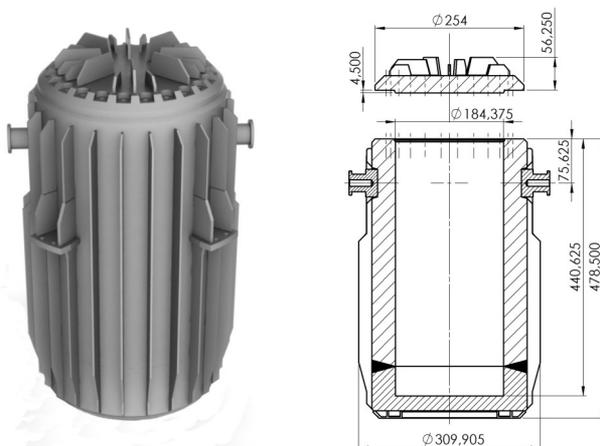
Fig. 10. Model of container for drop and pressure tests.
