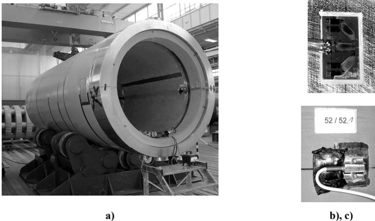
**Fig. 7.** a) body of container with installed strain-gages, b) strain-gage, c) sensor of acceleration [8].
