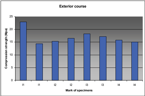
Fig. 4. Layer (course) I – compression tests.
