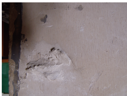
Fig. 2. The outdoor side of gypsum block after five year of exposition to Prague exterior weather conditions.
