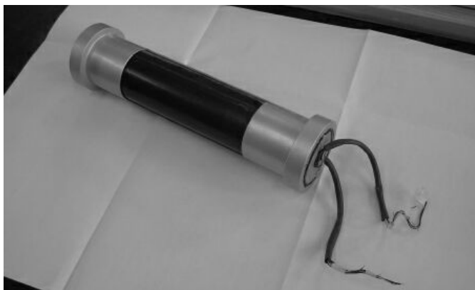
Fig. 11. Test piece manufactured with the use of the RTM technology, with ducts from strain gauges located on the inner surfaces of the metal parts.
