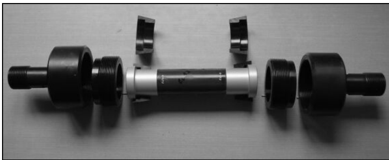
Fig. 4. Test piece, “double-root” type, for testing the static strength of the joint.
