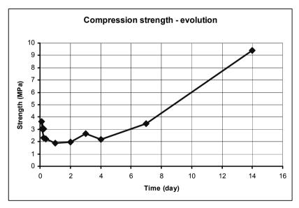
Fig. 2. Evolution of compression strength of gypsum.
