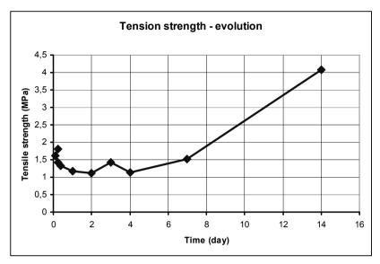
Fig. 3. Evolution of tensile strength of gypsum.
