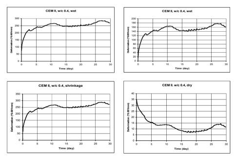
Fig. 2. Creep of specimens from cement paste w/c 0.4 (CEM II).
