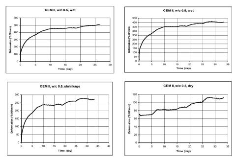
Fig. 3. Creep of specimens from cement paste w/c 0.5 (CEM II).
