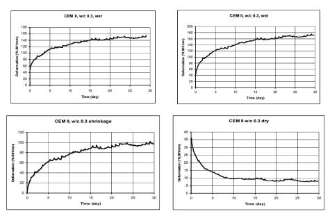
Fig. 1. Creep of specimens from cement paste w/c 0.3 (CEM II).
