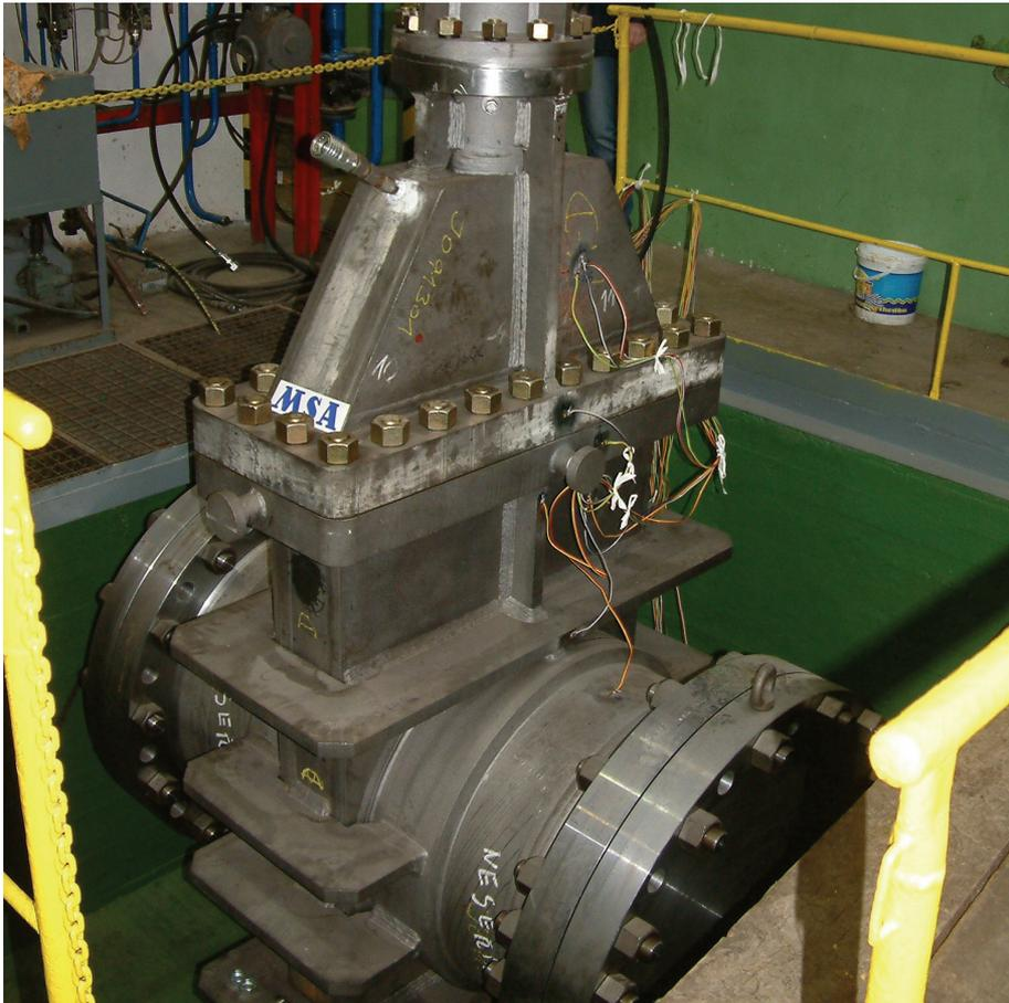
Fig. 2. Welded plate valve.
