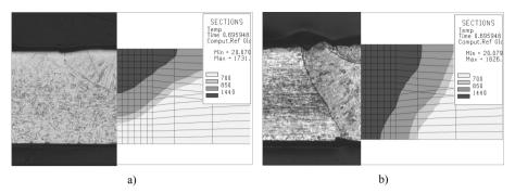
Fig. 4. Modelled and real weld cross section shape, a) sample no. 1, b) sample no. 2.
