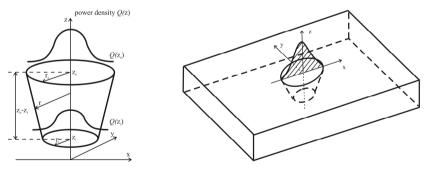
Fig. 2. Gaussian heat source applied to the material.
