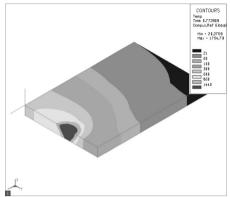
**Fig. 7.** Contours image of temperature field distribution in 0.772989 s time point.
