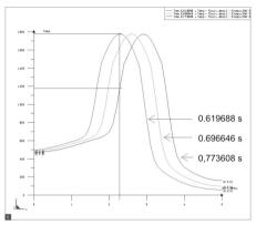
**Fig. 6.** Temperature – weld trajectory dependence for three different time points.
