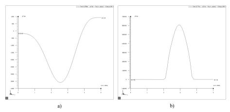
Fig. 8. Temperature rate along the welding trajectory for time point a) 0.76941 s, b) 0.77011 s.
