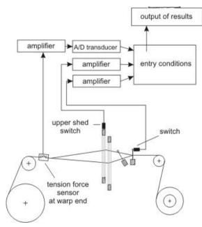
Fig. 4. Measurement scheme.
