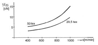
Fig. 2. Example weaving velocity dependence of force.
