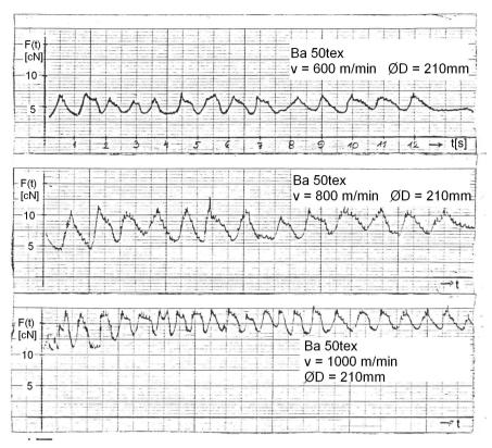
Fig. 1. Example output of electronic measurement result.
