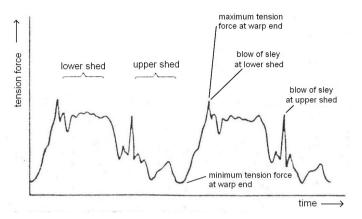
Fig. 3. Example time behaviour of tension force.
