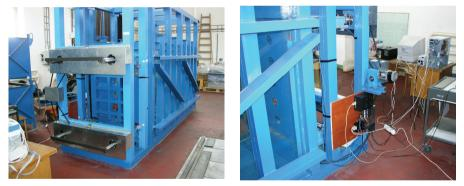
Fig. 2. a) (Left) Overall view of the computer-controlled front wall motor drive after the first development part and restructure of the moved front wall. The motor is on the left; the linear incremental position pick-ups near the skids cannot be seen. b) (Right) Motor drive in detail with hardware and computer behind.
