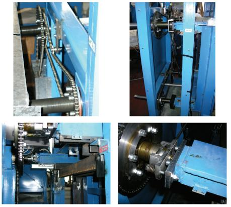
**Fig. 3. a)** (Above left.) Detail of upper screws and driving chain system (the motor is right down) in 31.7.2006. **b)** (Above right) Detail of upper screws for front wall movement with skids and linear incremental position pick-up (left side view in 19.9.2006) and **c) d)** (Below - views above and down resp.) after the development in Apr.2007 due to the rupture of the little plate off very hard steel under a bearing steel globe (Pictures in 4.6.2007.).
