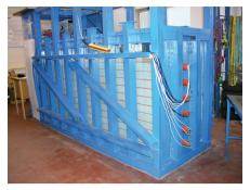
**Fig. 4.** Views of the solid back wall with six pressure sensors placed in and with the sample into.
