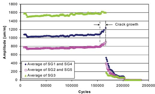
Fig. 10. Strain amplitudes recorded during fatigue test.
