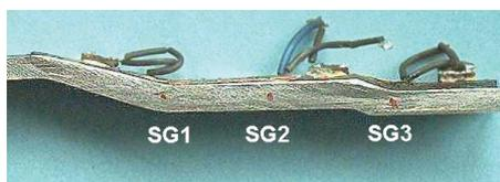
Fig. 5. Tube thickness on longitudinal cut.
