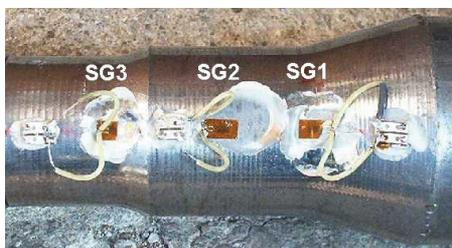
Fig. 4. Position of strain gauges.
