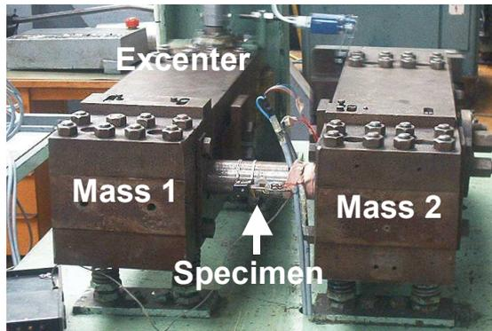
Fig. 1. Machine resonance system with masses and tested specimen as a springy element.
