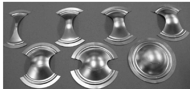
Figure 8. Different specimen geometries, from the entire blank to strongly waisted blanks
