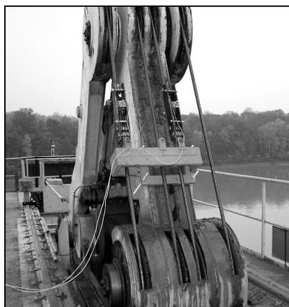
**Figure 1:** Force scanning in the lifting and closing cables
