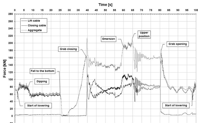
**Figure 2:** Dredger working cycles (forces in individual cables and their summation)
