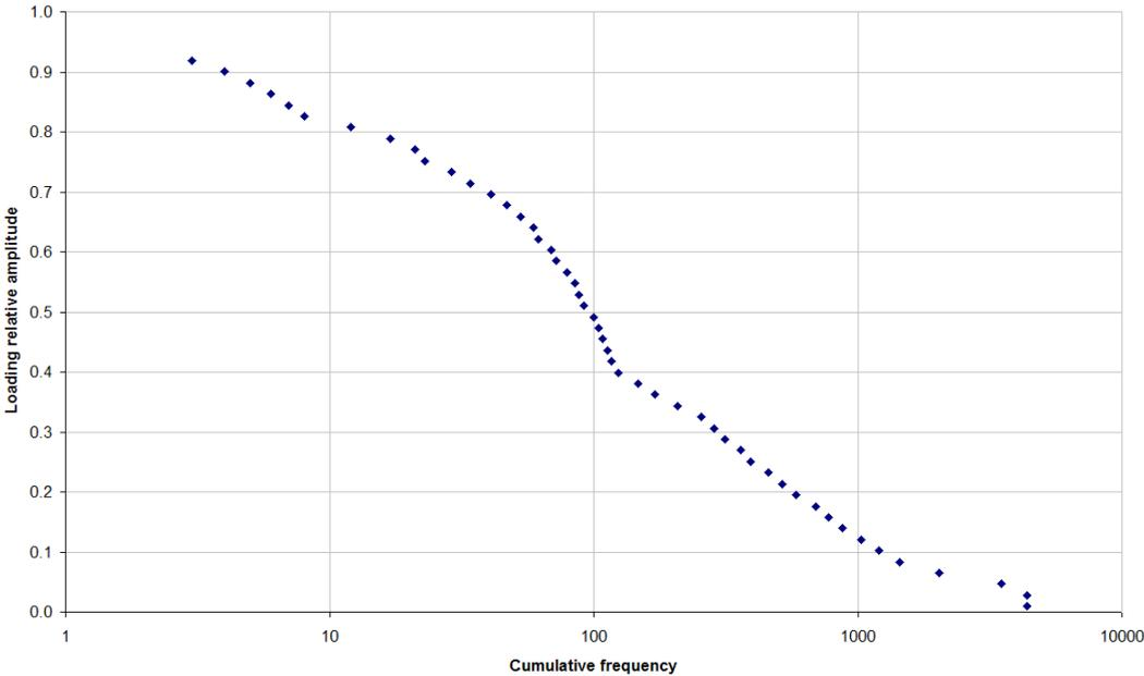
**Figure 4:** Dependence of loading relative amplitude on cumulative frequency
