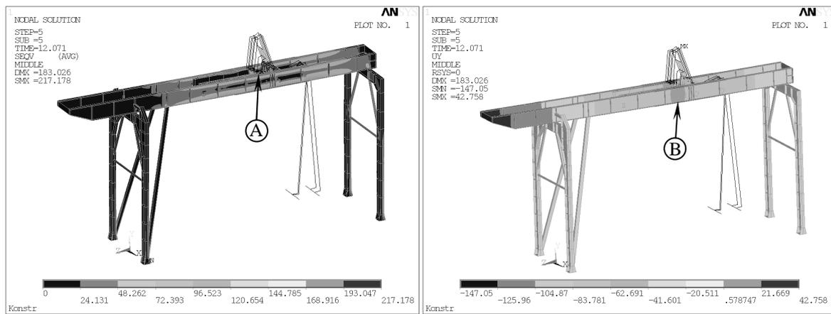
**Figure 7:** Dynamic calculation of the crane structure and points of the stress values pick-up (on the left) and nodal displacements in the direction of axis y (on the right).
