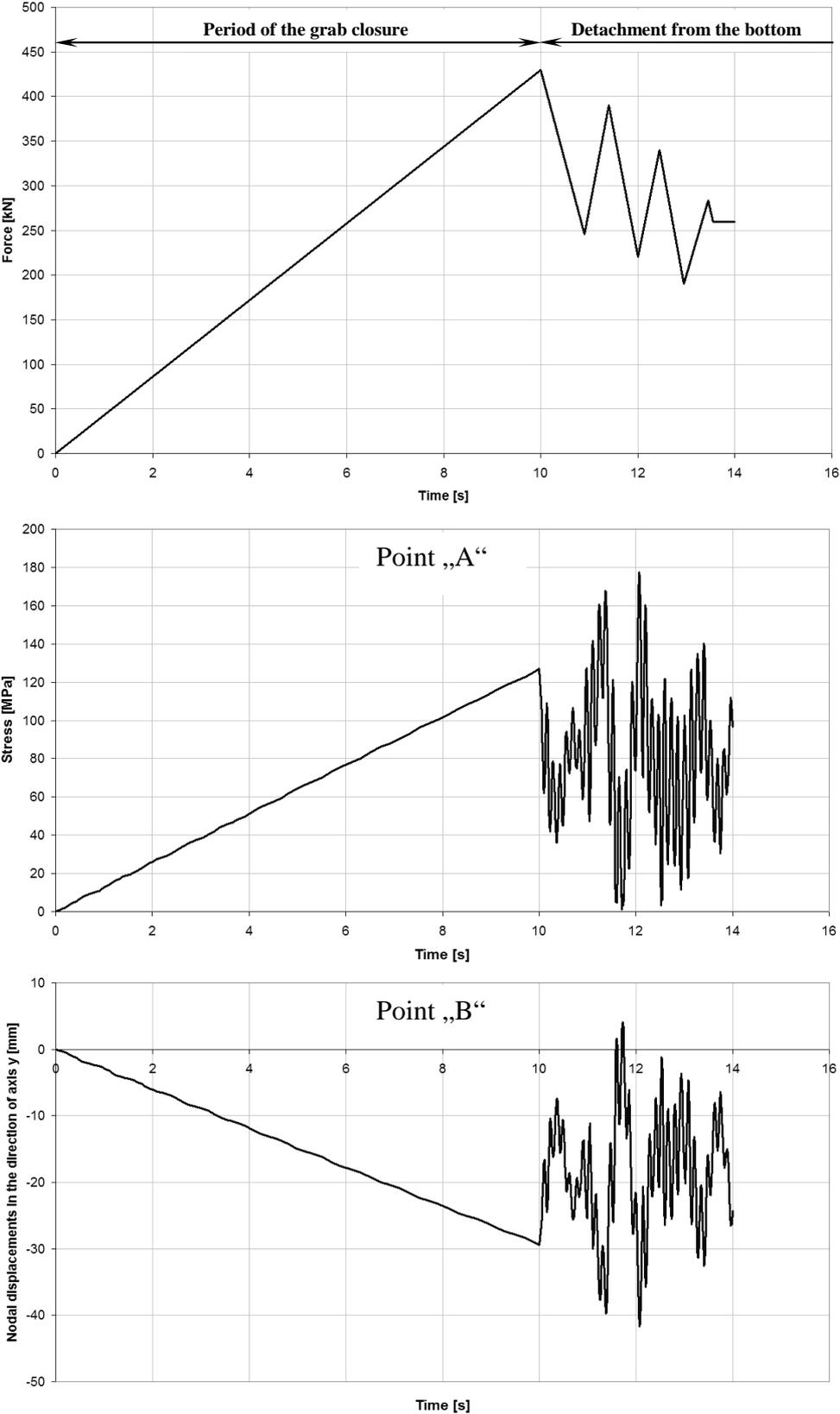
Figure 6: Dynamic calculation – loading force, stress and nodal displacements in selected points of the structure
