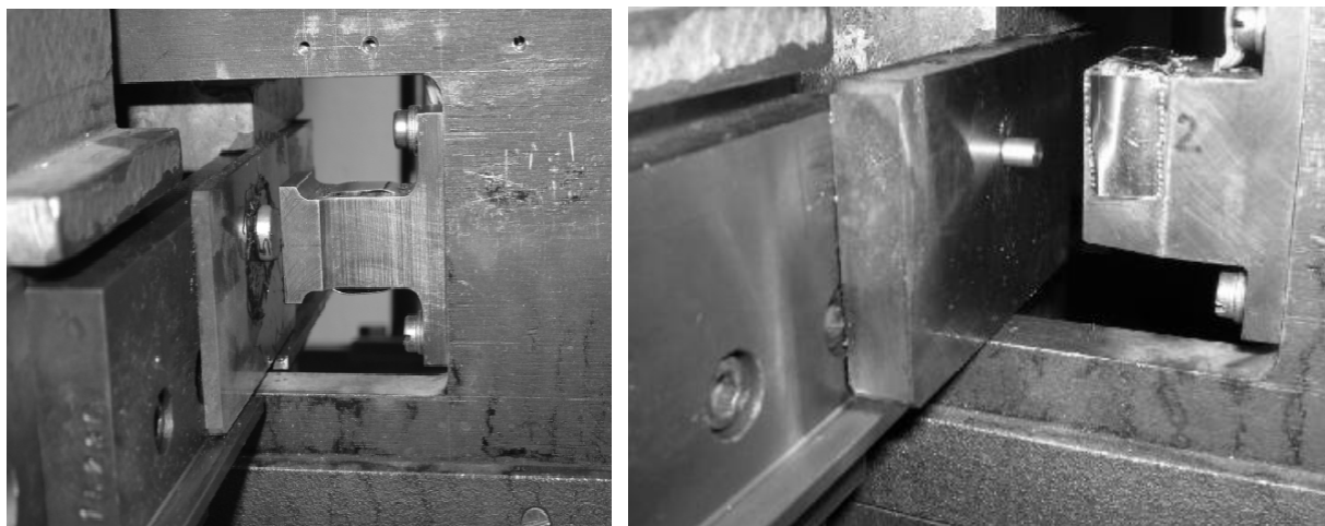
Figure 2: Tip of the instrumented impact hammer striker for dynamic compression testing.
