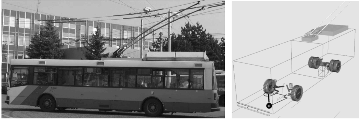
Figure 7: The ŠKODA 21 Tr low-floor trolleybus – a real vehicle and a multibody model visualization in the SIMPACK simulation tool.
