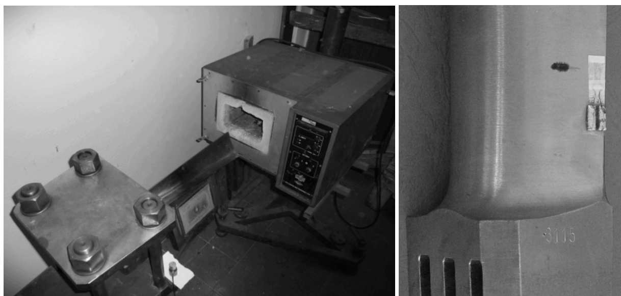
Figure 5: Workplace for fatigue testing of rotating machines blades under higher temperatures and the tested blade detail.
