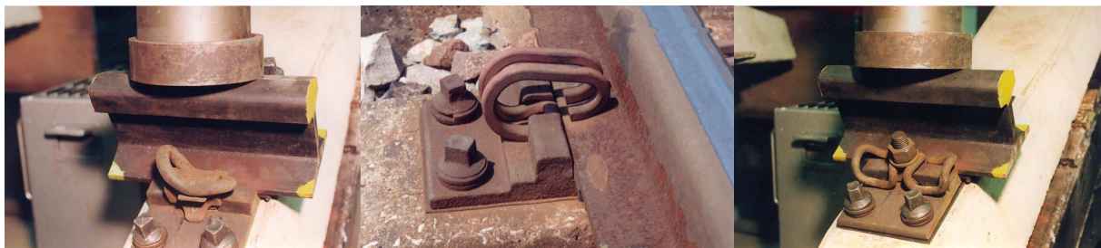
Figure 1: The experimentally tested tension clamps PANDROL, EWEM and SKL
