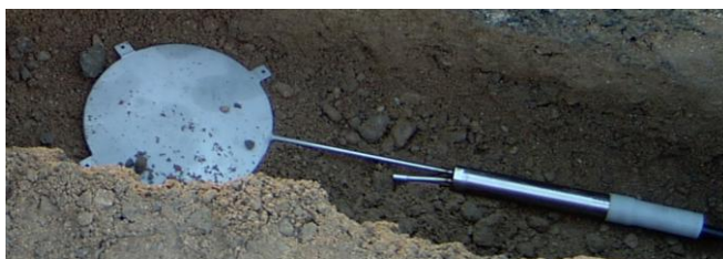
Fig. 2 Pressure sensor placed into railway substructure
