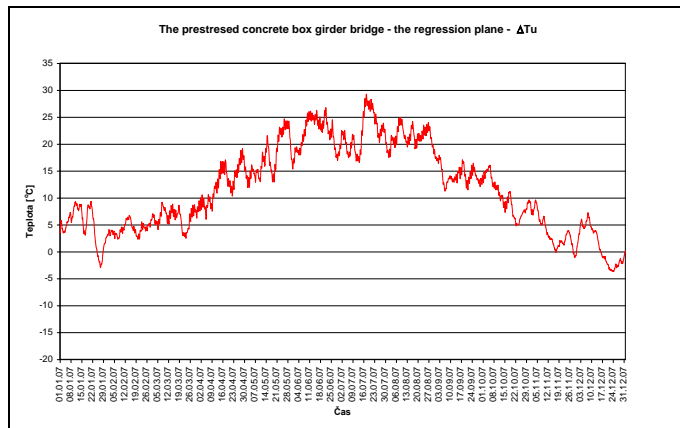
Fig. 2 Course of a uniform component of temperature \Delta T_u on the bridge during the year 2007
