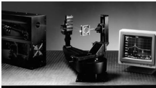
Fig. 3 Complete Angle Scatter Instrument. Laser source (left), detector (middle).
