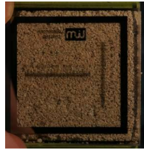
Fig. 2 Specimen n.2 in compression test, left, pixel calibration with glass gauge, right.
