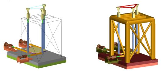
Fig. 1 Two models of platform in MSC.ADAMS software
