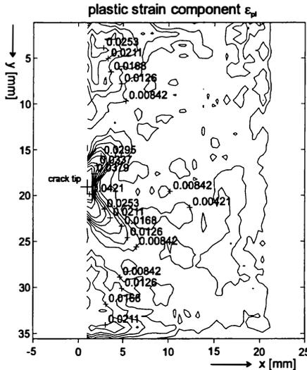
Fig.6.: Plastic strain component of equivalent strain.
