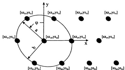
Fig.2: Deformed hexagonal points grid
