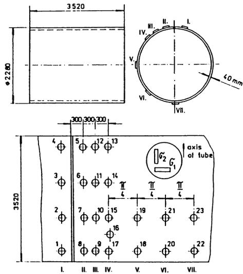
Fig.5 Layout of points for strain-gauge measurements on furnace steel centering.
