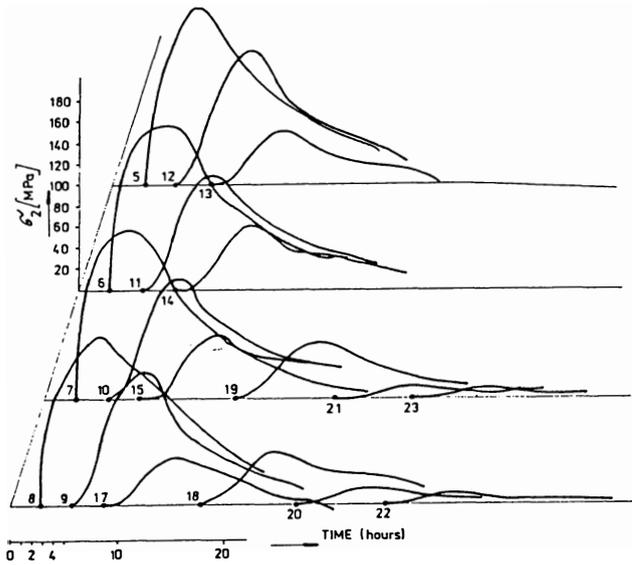
Fig.7 Stress pattern  $\sigma_2$  at distance of 300 mm from axis of steel centering weld.
