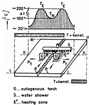
Fig.8 Functional chart of portable device for local heating with water spray.
