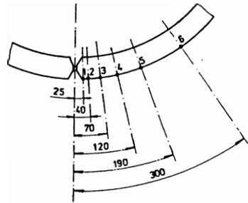
Fig.2 Layout of thermo-electric couples.
