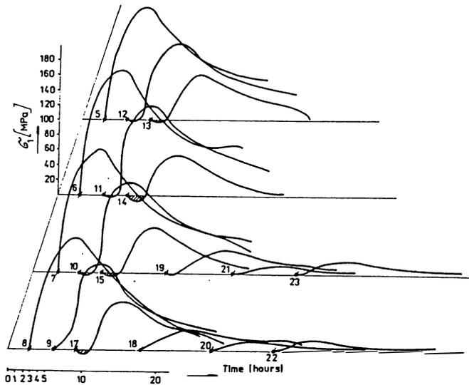
Fig.6 Stress pattern  $\sigma_1$  at distance of 300 mm from axis of steel centering weld.
