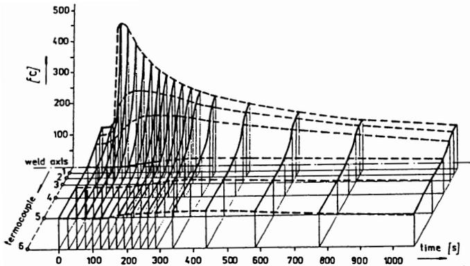
Fig.4 Field of temperature in surroundings of weld, last layer (last cover layer of outer weld).
