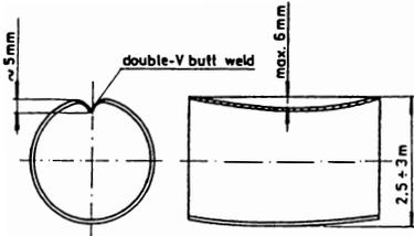
Fig.1 Example of shape and size of steel centering deformation.
