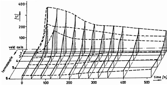
Fig.3 Field of temperature in surroundings of weld at welding of 1st layer of weld (internal side of double V butt weld).
