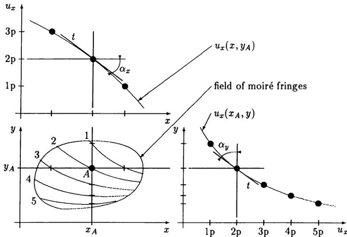
Figure 3: Displacement curves and strain components
