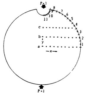
Fig. 3-Separation of stress in a disk 44 elements/44 nodes.
