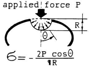
Fig. 2- Boundary condition for an isolated force.
