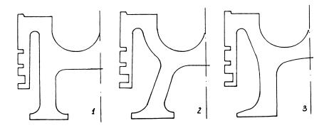
Fig.1. The versions of a nodal cast iron piston, tested by using photoelasticity.
